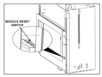
Figure 2.4 Location of Module Reset Switch - Tonic Front
